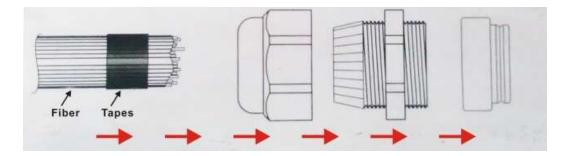
3. Cut the fibre bundle to a flat surface with a heat-knife or blade.
