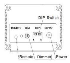
The light engine can be programmed with the combination of the DIP switches at the back of the unit and the remote controller. The two control methods complement each other. Some functions can be set by the DIP switches only, while others, by the remote controller.
